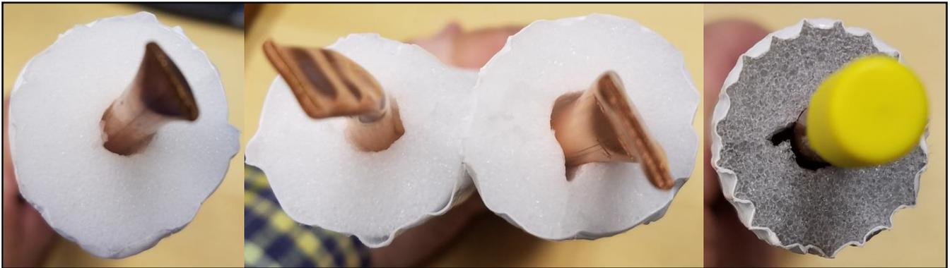
Figure 2: Examples of gaps at the termination ends of polyethylene linesets
